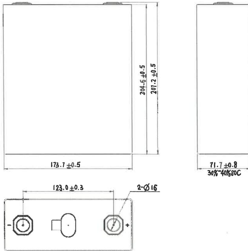
Fig. 9 Diagram of cell size and appearance
