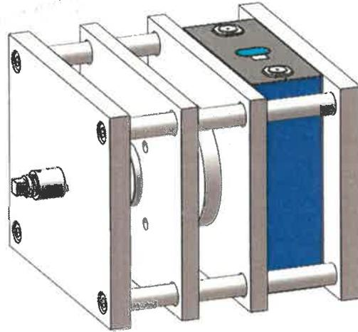
Fig. 5 Diagram of cell with swelling force clamp
