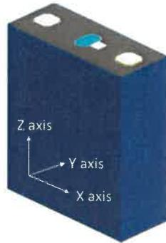
Fig. 8 Diagram of LF280K cell direction
