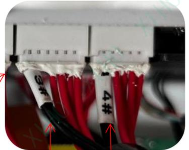
**Connection Note:** Ensure the black numbered cable is on the LEFT. Incorrect orientation will short-circuit and permanently damage the PCB board.
